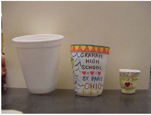
FIGURE 1 Polystyrene cups predeployment (left), after being deployed to 95 m in Lake Superior (center), and after deployment to approximately 250 m in the Atlantic Ocean (right) (color figure available online).
